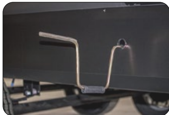
Slideout Override Access Hole & Crank Handle Extension
