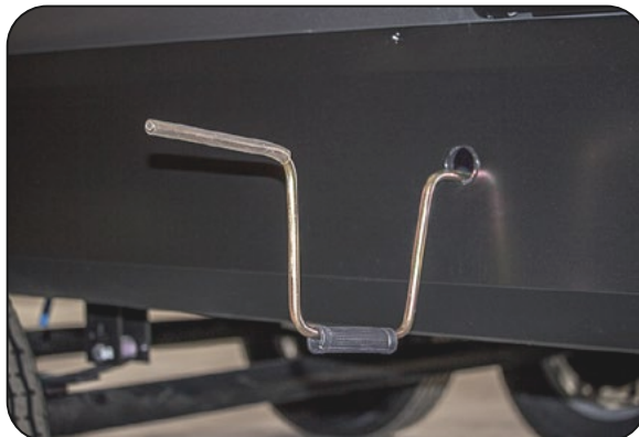
Slideout Override Access Hole & Crank Handle Extension
