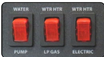
Water Pump & Water Heater On/Off Switches
