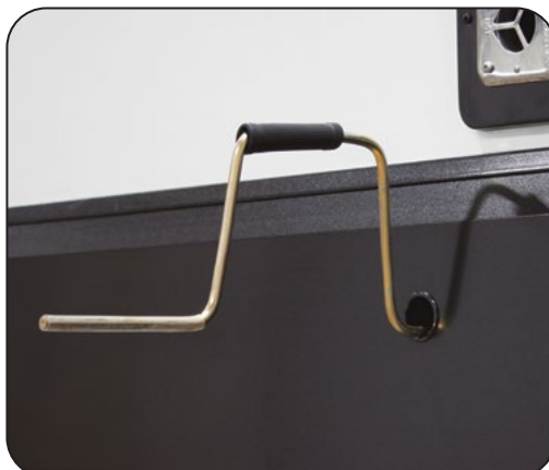
Slideout Override Access Hole & Crank Handle Extension
