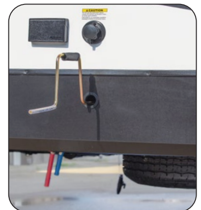
Spare Tire Access Hole & Crank Handle Extension
