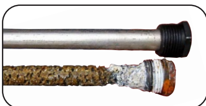
Brand New Anode Rod (top) Corroded Anode Rod (bottom)
