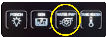
Water Pump On/Off Switch
