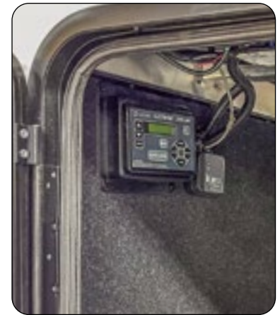
The Ground Control 3.0 LCD Touch Pad is located inside of the off-door side, forward compartment
