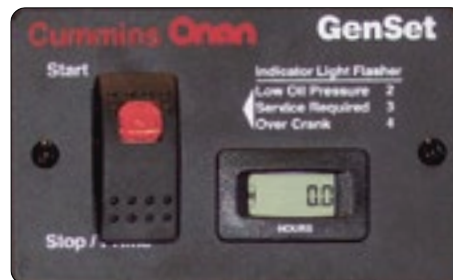
The Generator Remote Switch is found on the Command Center
