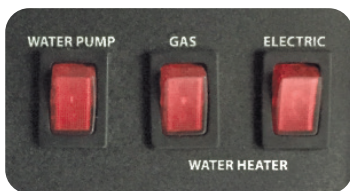
Water Pump & Water Heater On/Off Switches
