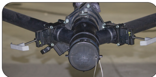
Sewer Outlet Connection Is Located Under the RV on the Off-Door Side
