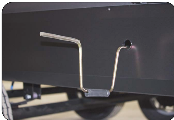
Slideout Override Access Hole & Crank Handle Extension
