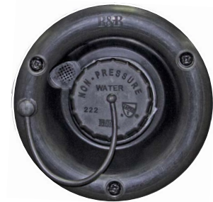
Fresh Water Gravity Fill Inlet
