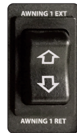
The Patio Awning Switch is located inside the RV, on the Command Center.
