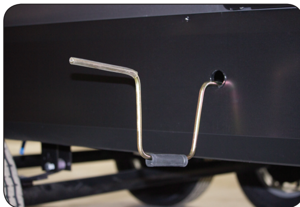
Slideout Override Access Hole & Crank Handle Extension
