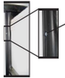
Step 1 – Typical Schwintek motor retention screw location, viewed from inside the RV.
