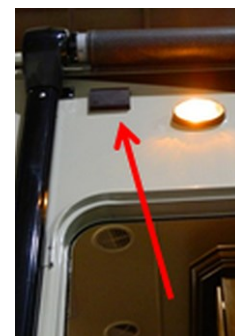
Arrow points to typical awning accessories plug (not available on newer units).
