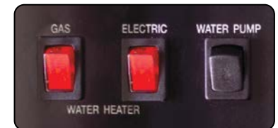
Water Pump & Water Heater On/Off Switches
