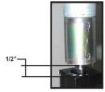
Step 3 – Typical Schwintek motor, disengaged.
