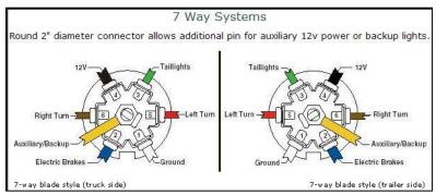
Typical 7-way wire harness wiring diagram
