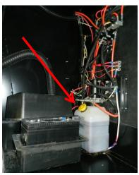
Typical reservoir for both the hydraulic landing gear and hydraulic slide system, it is located in the front-facing compartment. The red arrow points to the breather/fill cap.
