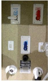
valve positions for Typical sanitization (connect hose to white city water fill inlet, located to the left of the white sewer tank flusher water inlet).
