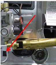
If the water heater does not work, make sure the power switch (indicated by the red arrow, located by removing the exterior water heater door) was not inadvertently switched OFF.
