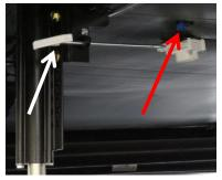
The white arrow indicates the fresh tank drain valve. The red arrow indicates the fresh water drain location (valve & drain locations vary by model).
