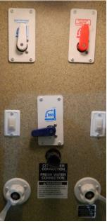
Typical valve positions for winterization (connect hose to white city water fill inlet, located to the left of the white sewer tank flusher water inlet).
