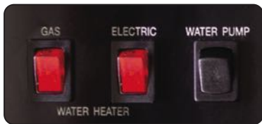
Water Pump & Water Heater On/Off Switches
