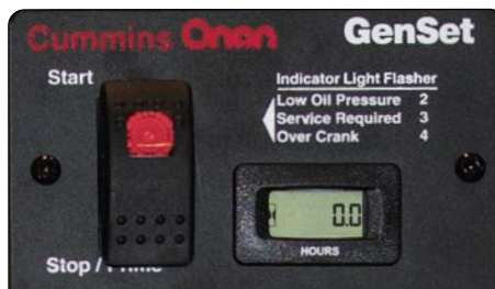
The Generator Remote Switch is found on the Command Center
