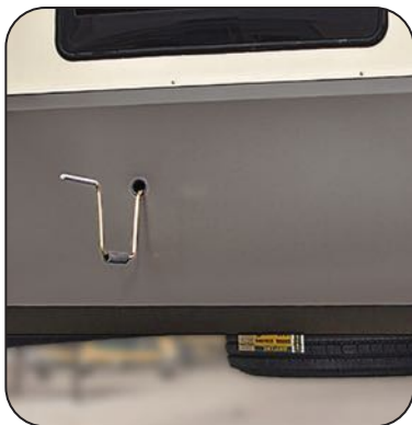
Spare Tire Access Hole & Crank Handle Extension
