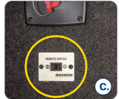
Inverter Remote Switch
