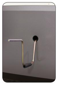
Slideout Override Access Hole & Crank Handle Extension
