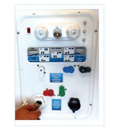
It is normal for some winterizing solution to exit inlet as hose is being disconnected.
