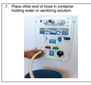
8. Push **"PUMP"** switch so that the light on switch is lit.
