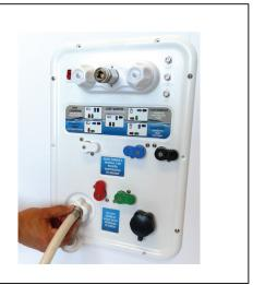
7. Turn water on. Fresh water tank should begin to fill.
