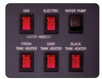
Water Pump & Water Heater On/Off Switches
