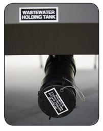
Sewer Outlet Connection Is Located on the Off-Door Side
