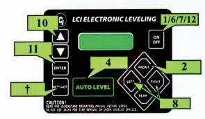
1. Press "On/Off" button to turn panel on (display reads "JACKS UP").
