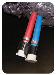
Low-Point Drains located under the RV
