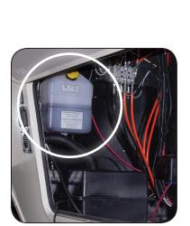
The Hydraulic Fluid Reservoir is located in the Front Compartment. It supplies fluid to both the Hydraulic Landing Gear & the Hydraulic Slide Systems.
