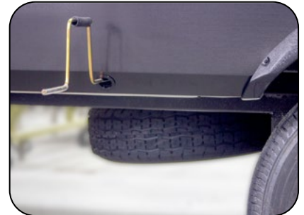
Spare Tire, Access Hole & Crank Handle Extension
