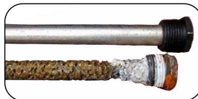
Brand New Anode Rod (top) Corroded Anode Rod (bottom)
