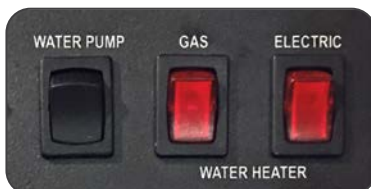
Water Pump & Water Heater On/Off Switches
