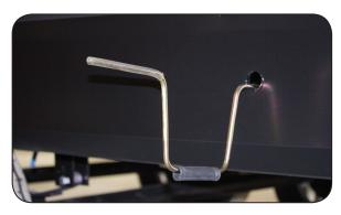
Slideout Override Access Hole & Crank Handle Extension
