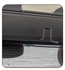
Spare Tire, Access Hole & Crank Handle Extension
