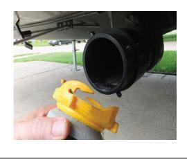
2. Open black waste holding tank valve and leave open. Allow tank to drain.
