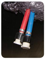
Low-Point Drains located under the RV
