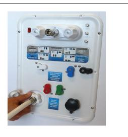
7. Turn "on" water at the source. Water should be available to all fixtures.
