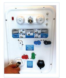
It is normal for some winterizing solution to exit inlet as hose is being disconnected.
