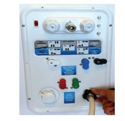
4. Fully open faucet at water supply source (40 psi minimum) flushing tank until water appears clear in 4" discharge hose.
