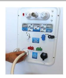
7. Place other end of hose in container holding water or sanitizing solution.
