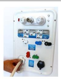
7. Turn water on. Fresh water tank should begin to fill.
