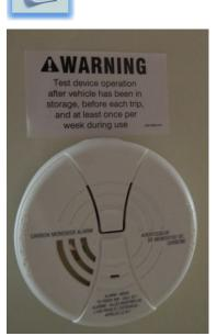
Typical carbon monoxide (CO) alarm and label.
