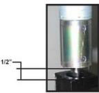
Step 3 – Typical Schwintek motor, disengaged.
