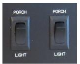
*Typical exterior light switches, located in the command center:*
