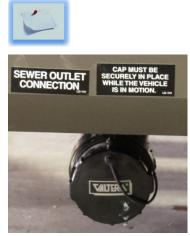
*Typical sewer outlet connection, located on the off-door side.*
