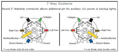
Typical 7-way wire harness wiring diagram
