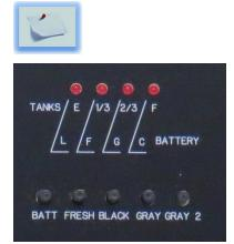
Photo shows a typical monitor panel section, located on the command center inside the RV.
