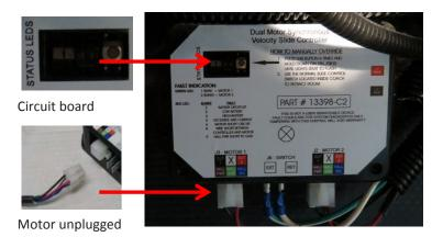
Typical Schwintek slide controller, located in the front facing compartment of your FW.
