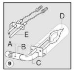
Typical Atwood burner tube assembly
