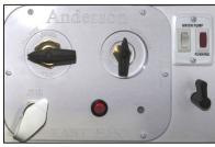
*Close-up of typical fresh water connections, located in the utility center*
