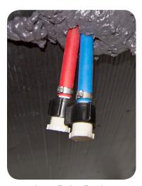
Low-Point Drains located under the RV
