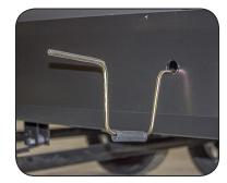
Slideout Override Access Hole & Crank Handle Extension
