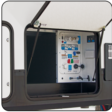
The Nautilus P1 Water Control System Is Located On The Forward Off-Door Side.
