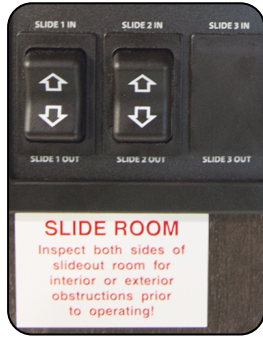
The Slide Room Switches are located inside the RV, on the Command Center.
