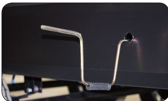
Slideout Override Access Hole & Crank Handle Extension
