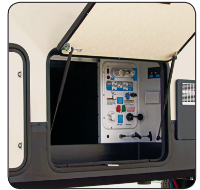
The Nautilus P1 or P2 System Is Located in the Forward, Pass-Thru Storage on the Off-Door Side.
