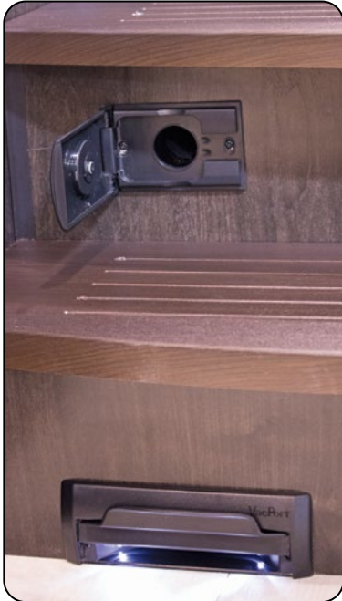
The Central Vacuum Hose Inlet & Toe Kick are located inside the RV, by the front stairs on most floorplans.
