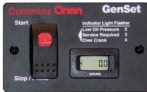
Generator Remote switch is found on the Command Center
