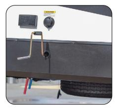
Spare Tire Access Hole & Crank Handle Extension
