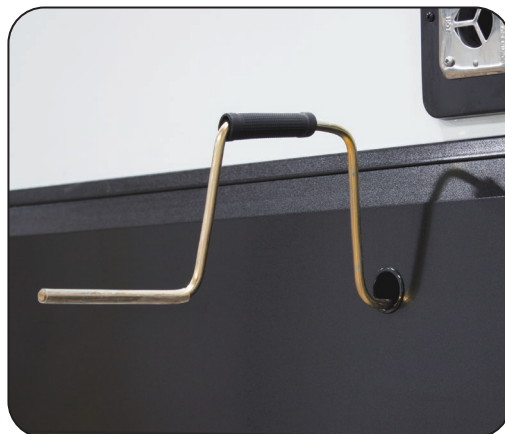
Slideout Override Access Hole & Crank Handle Extension
