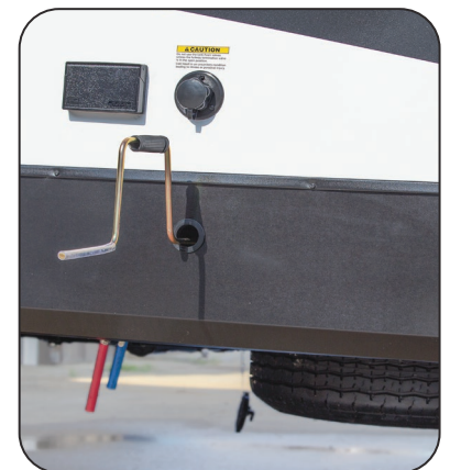
Spare Tire Access Hole & Crank Handle Extension
