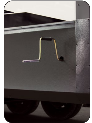
Spare Tire Access Hole & Crank Handle Extension
