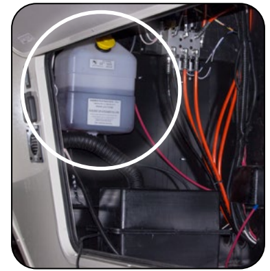
The Hydraulic Fluid Reservoir is located in the Front Compartment.
