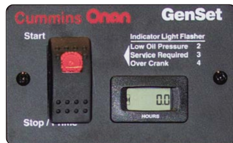
On the G-Class, the Generator Remote Switch is found on the Command Center
