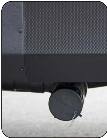
Sewer Outlet Connection Is Located Under the RV on the Off-Door Side
