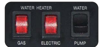
Water Heater & Water Pump On/Off Switches
