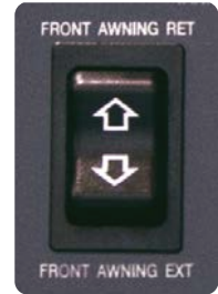
On the G-Class, the Patio Awning Switch is located inside the RV, on the Command Center.
