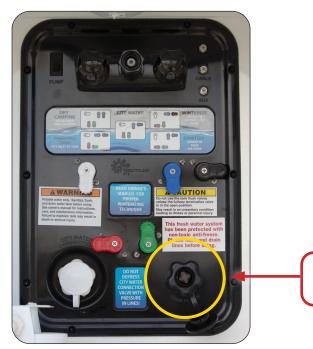
Black Tank Flusher or *Tank Flush Inlet*
