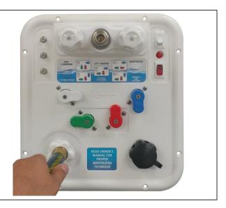
3. Place other end of hose in container holding water or sanitizing solution.
