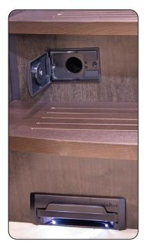
The Central Vacuum Hose Inlet & Toe Kick are located inside the RV, by the front stairs on most floorplans.
