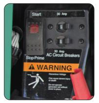
Generator main power & circuit breaker switches.
