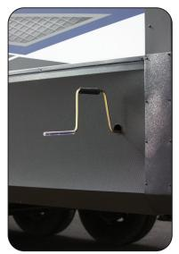
Spare Tire Access Hole & Crank Handle Extension
