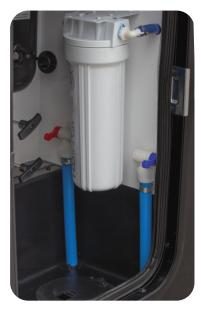
Low-Point Drains are located in the Universal Docking Station
