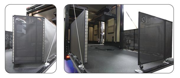
4. Slide the railing onto the keeper bases and lock in place.
