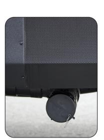
Sewer Outlet Connection Is Located Under the RV on the Off-Door Side
