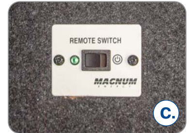
Inverter Remote Switch
