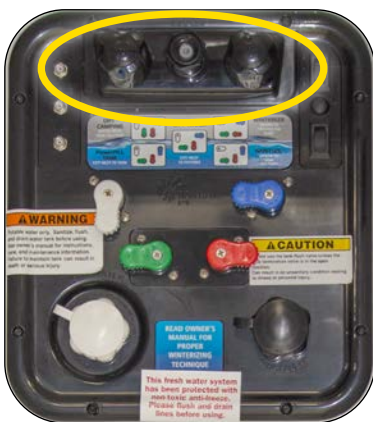
Exterior Spray Port
