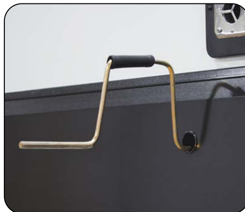
Slideout Override Access Hole & Crank Handle Extension
