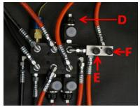
Typical hydraulic slide rooms override valves, generally located in the front facing compartment of the Solitude 369RL.
