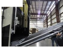
2a. Carefully lower and open the ramp door making sure both ramp door cable ends are fastened securely...
