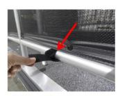
7. Remove the velcro straps (TIP: re-wrap them on the gates to ensure they aren't lost) that secure the end patio gates shut in the travel position.
