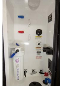
Close-up of a typical utility center with the Alternative Valve System.
