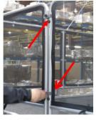
8b. ...then screw the top and bottom locks in as shown to secure the end gates in the closed (locked) position.
