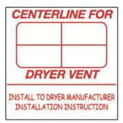
Dryer vent installation label, typically located inside the off-door side front bedroom closet.
