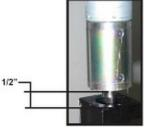
Step 3 – Typical Schwintek motor, disengaged.
