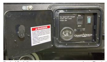
Typical fuel dispensing system emergency shut off switch hatch
