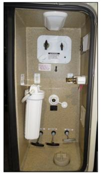
Close-up of a typical utility center with the Anderson-Kantleak system.
