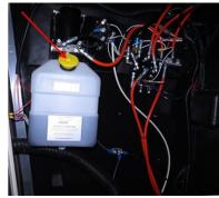
Typical reservoir for both the hydraulic landing gear and hydraulic slide system, it is located in the front-facing compartment. The red arrow points to the breather/fill cap.
