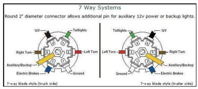
Typical 7-way wire harness wiring diagram
