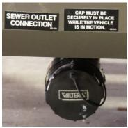
Typical sewer outlet connection, located on the off-door side.
