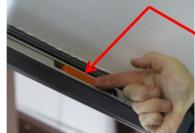
Locate both orange colored locking mechanisms at the top inside of the extended awning, and pull the handles towards you (as shown above) to release the retractable legs.
