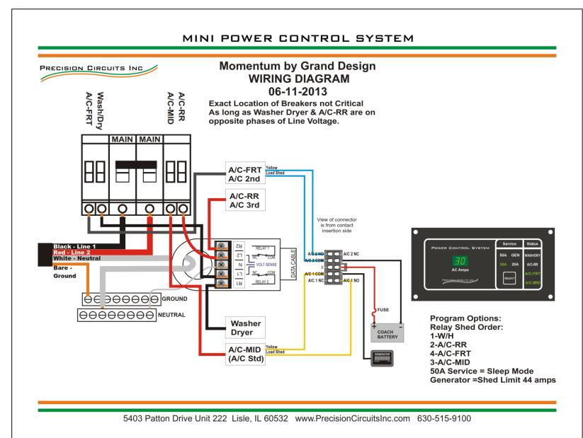
Diagram shows the typical layout for the Mini-EMS
