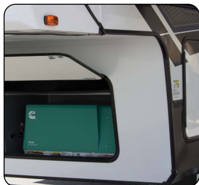
Generator (if so equipped) is located in the front compartment of your RV.
