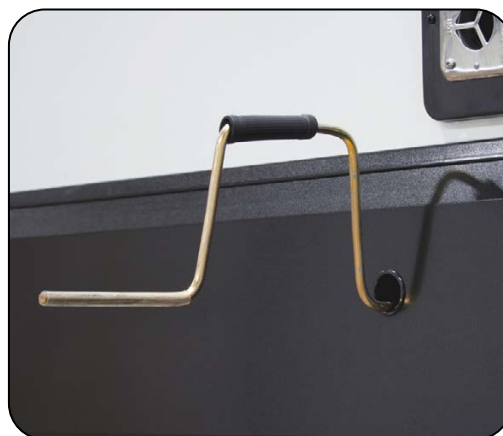
Slideout Override Access Hole & Crank Handle Extension
