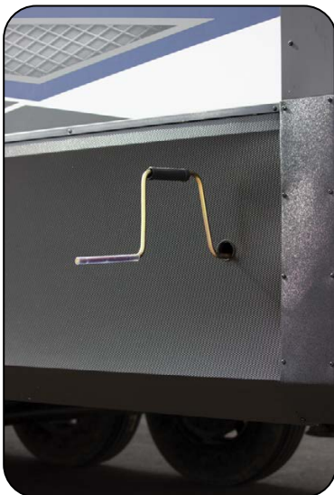
Spare Tire Access Hole & Crank Handle Extension
