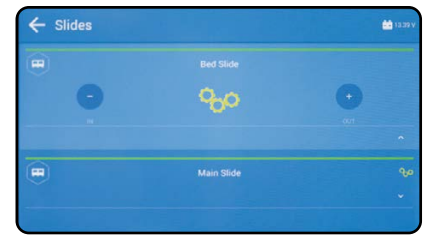
The Slide Room controls are found on the ONEControl® System.
