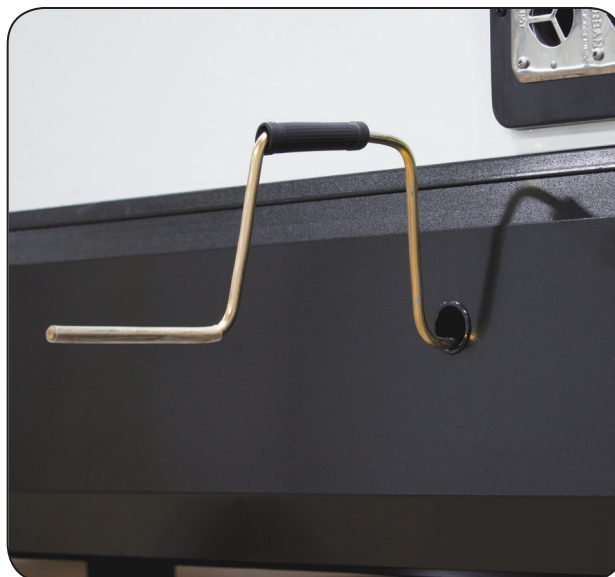
Slideout Override Access Hole & Crank Handle Extension
