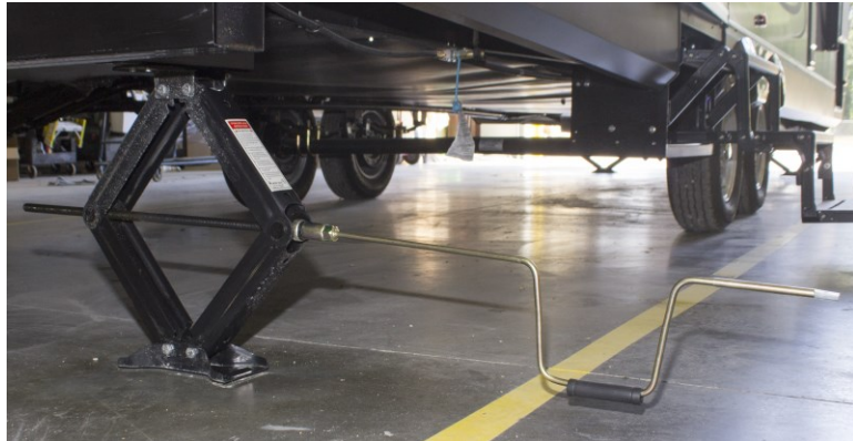
Typical stabilizer jacks (shown in the extended position), with the supplied crank handle attached
