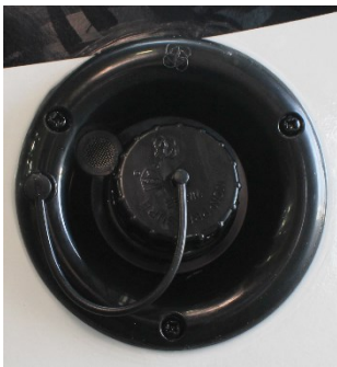
Typical gravity water fill inlet
