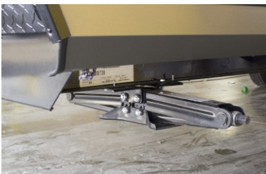
Typical stabilizer jack, shown retracted in the travel position.
