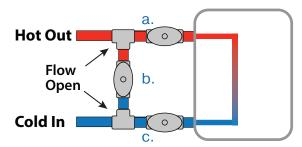
Draining the Water Heater - Valve Positions
