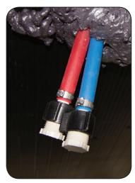
Low-Point Drain Valves located under the RV
