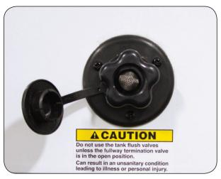
Black Tank Flusher Inlet is located on the off-door side of the RV.
