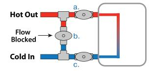
During winterization/sanitization, turn the water heater bypass valves to the **bypass** position shown below:
