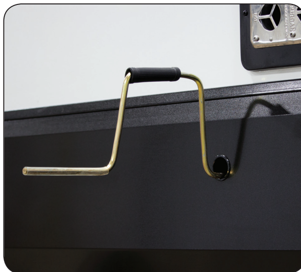
Slideout Override Access Hole & Crank Handle Extension
