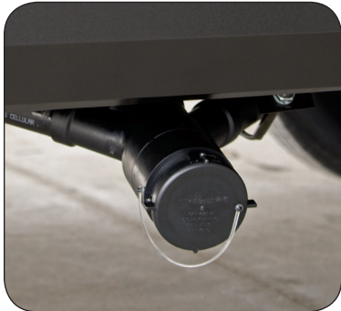
Sewer Outlet Connection Is Located Under the RV on the Off-Door Side
