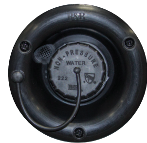
Fresh Water Gravity Fill Inlet
