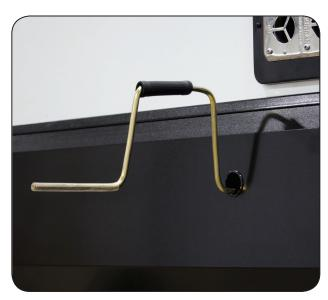
Slideout Override Access Hole & Crank Handle Extension
