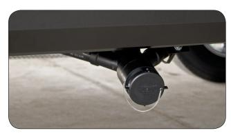
The Sewer Outlet Connection is located under the RV. on the off-door side.
