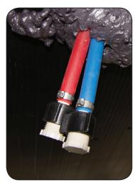
Low-Point Drain Valves located under the RV
