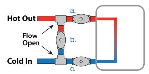
Draining the Water Heater - Valve Positions
