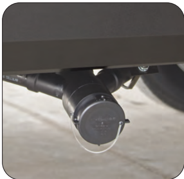
Sewer Outlet Connection Is Located Under the RV on the Off-Door Side
