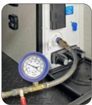
Air Compressor Hose with Pressure Gauge
