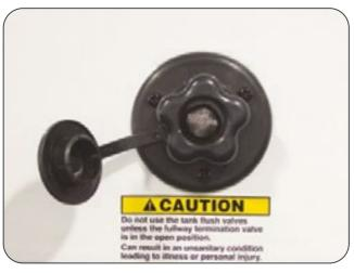
The Black Tank Flusher Inlet is located on the off-door side of the RV.
