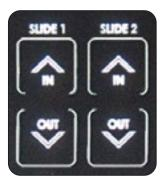
The Slide Room Switches are located inside the RV, on the Command Center.
