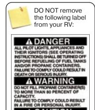
THES PROPANE PIPING SYSTEM IS DESIGNED FOR USE WITH PROPANE ONLY. DO NOT CONNECT NATURAL GAS TO THIS SYSTEM. Securely cap inlet when not connected for use. After turning on propane, except after normal cylinder replacement, test propane piping and connections to appliances for leakage with soapy water or bubble solution. Do not use products that contain ammonia or chlorine.
