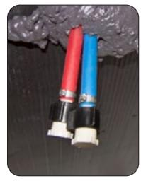
Low-Point Drain Valves located under the RV
