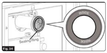
11. A sealing ring is assembled on the chimney. (*Fig. 34*) Inspect to make sure the seal does not have any cracks or breaks, and that it is in good condition. *Contact Furrion for replacement.*
