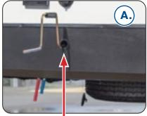
Spare Tire Access Hole & Crank Handle Extension
